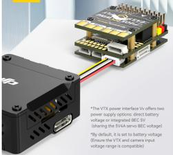
\*The VTX power interface Vx offers two power supply options: direct battery voltage or integrated BEC Vx. (Using the 5Vx option BEC voltage!)
