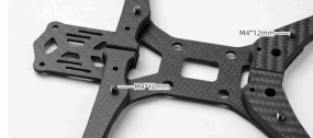
NO.2 Fix the middle plate, use M3*8mm to fix the frame protection plate below
