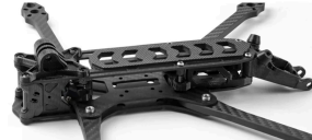
NO.6 Install the GoPro mount and the top plate
