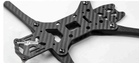
NO.3 Use M3*18, M3*20, M3*28 aluminum pillar to fix the position corresponding to the picture below
