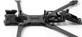
NO.6 Install the GoPro mount and the top plate
