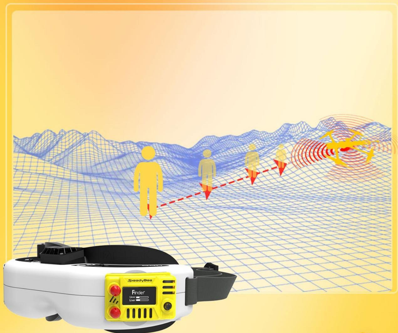
The Model Finder will display the real-time signal strength of the video transmission and emit a sound, guiding you to the direction where the signal gets stronger, allowing you to quickly locate your drone's position.
