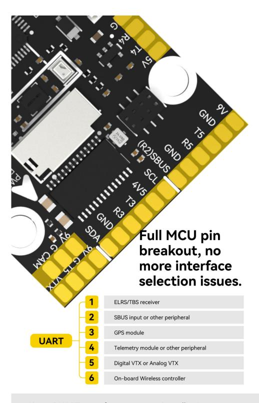
Up to 6 UART ports for easy expansion, allowing you to connect various external modules, from GPS to Digital VTX.
