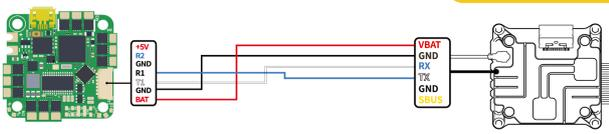
When not using the DJI remote controller, don't connect the S-BUS and GND.
