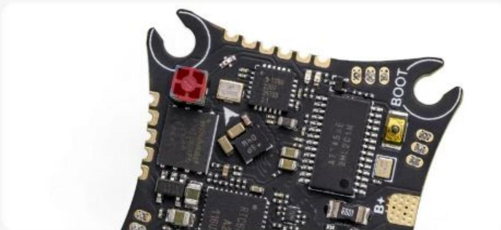
Built-in integrated 200mW 5.8GHz analog video transmission
