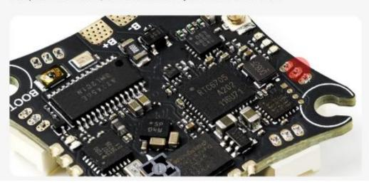
This is an ultra-light F411 5A 1S AlO integrated brushless flight controller, integrated SPI ExpressLRS 2.4G receiver, and integrated 200mW 5.8GHz adjustable power video transmission at the same time The SPI ELRS receiver uses patch ceramic antennas to solve the short-distance problem of the ancient SPI D8/D16 protocol. The ELRS receiver superimposes 200mW high-power video transmission to easily fly around the
