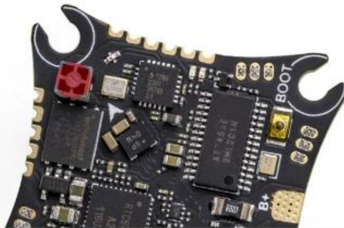
Built-in integrated 200mW 5.8GHz analog video transmission
