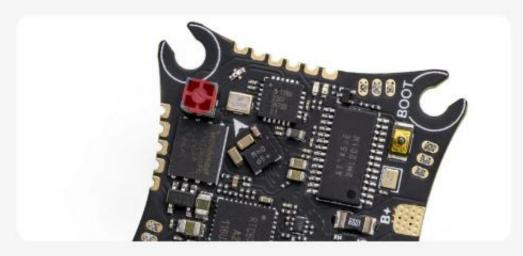
Built-in integrated 200mW 5.8GHz analog video transmission Fly around harsh indoor environments with ease
