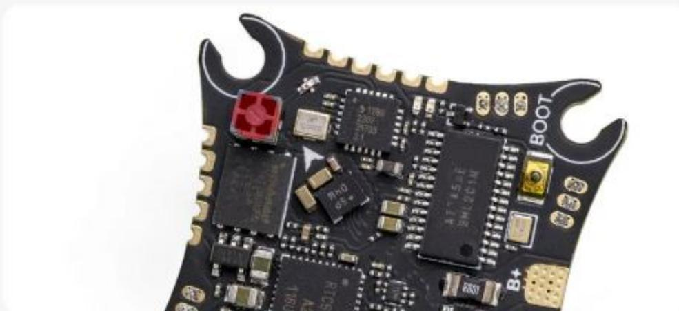
Built-in integrated 200mW 5.8GHz analog video transmission
