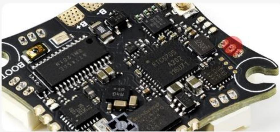
This is an ultra-light F411 5A 1S AIO integrated brushless flight controller, integrated SPI ExpressLRS 2.4G receiver, and integrated 200mW 5.8GHz adjustable power video transmission at the same time. The SPI ELRS receiver uses patch ceramic antennas to solve the short-distance problem of the ancient SPI D8/D16 protocol. The ELRS receiver superimposes 200mW high-power video transmission to easily fly around the
