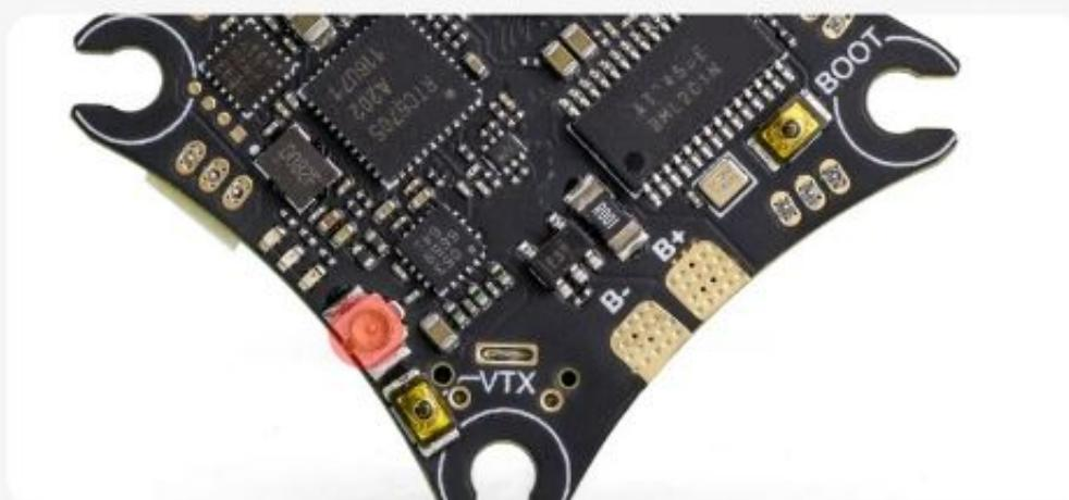
Independent 3P mount, which can be directly connected to the motor
