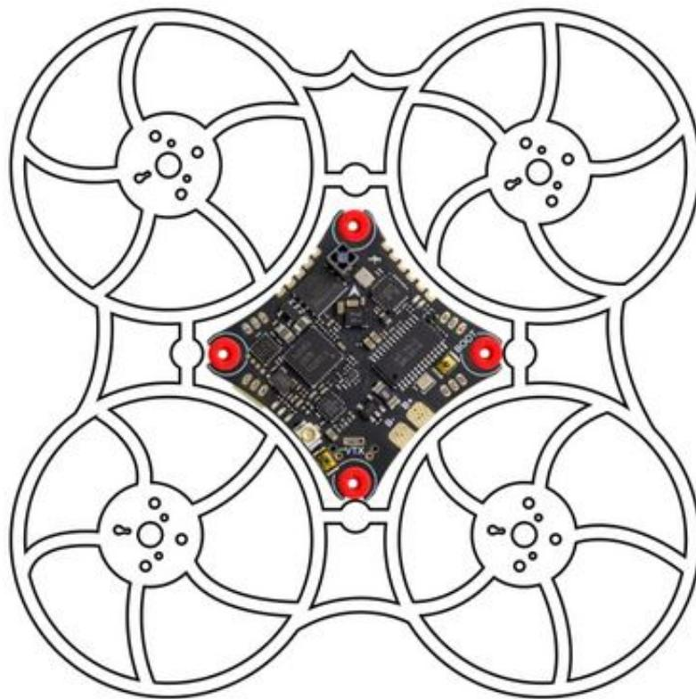
Integrated SPI ExpressLRS 2.4G receiver/external CRSF protocol receiver
